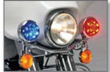
Optional 4" Round TIR6 Super-LED with extended lens
